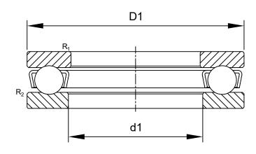
R<sub>1/2</sub>: min0.6 mm Chamfer Dimension Washer
