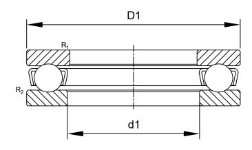
R<sub>1,2</sub>: min0.6 mm Chamfer Dimension Washer
