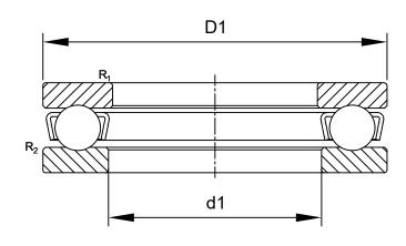
R<sub>1,2</sub>: min0.15 mm Chamfer Dimension Washer
