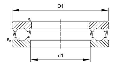
R<sub>1,2</sub>: min0.15 mm Chamfer Dimension Washer
