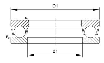
R<sub>1,2</sub>: min0.15 mm Chamfer Dimension Washer
