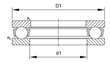
$R_{1,2}: \quad \text{min} \ 0.15 \quad \text{mm} \quad \quad \text{Chamfer Dimension Washer}$
