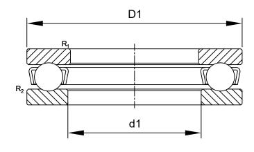
R<sub>1,2</sub>: min0.15 mm Chamfer Dimension Washer
