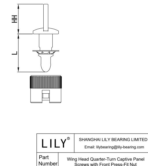
Wing Head Quarter-Turn Captive Panel Screws with Front Press-Fit Nut
