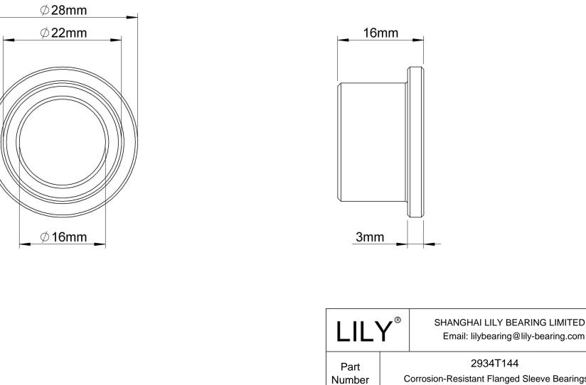
2934T144 Corrosion-Resistant Flanged Sleeve Bearings
