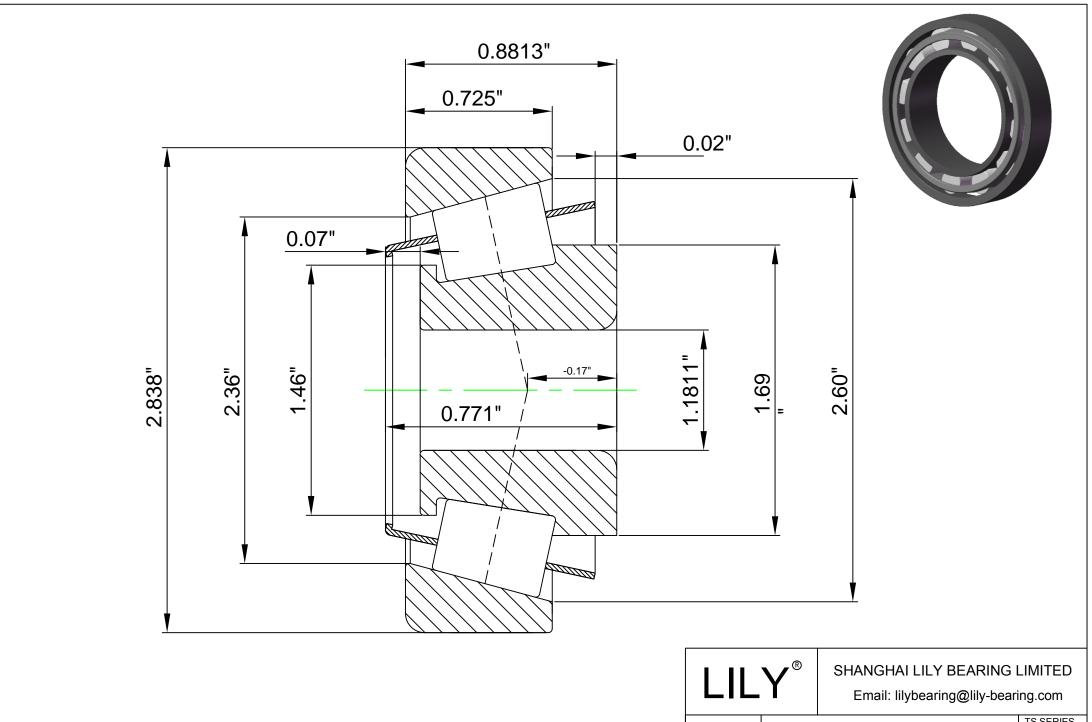
Part 14118A-14283(Tapered Single Roller Bearings) Number
